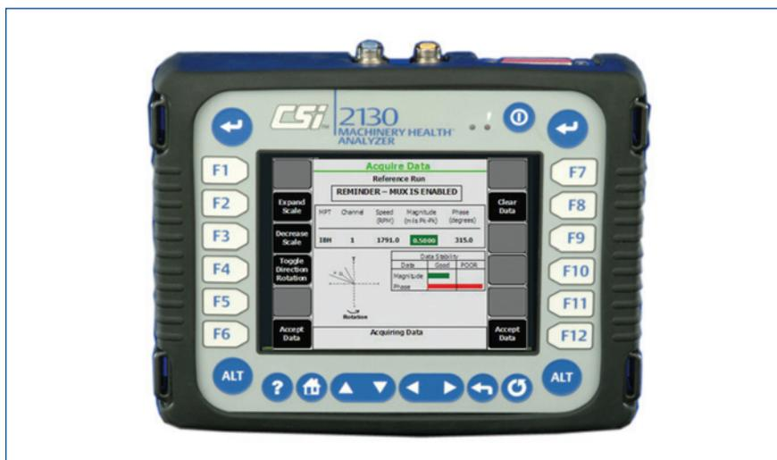
*The CSI 2130 Machinery Analyzer features an easy-to-use graphical balancing user interface.*
