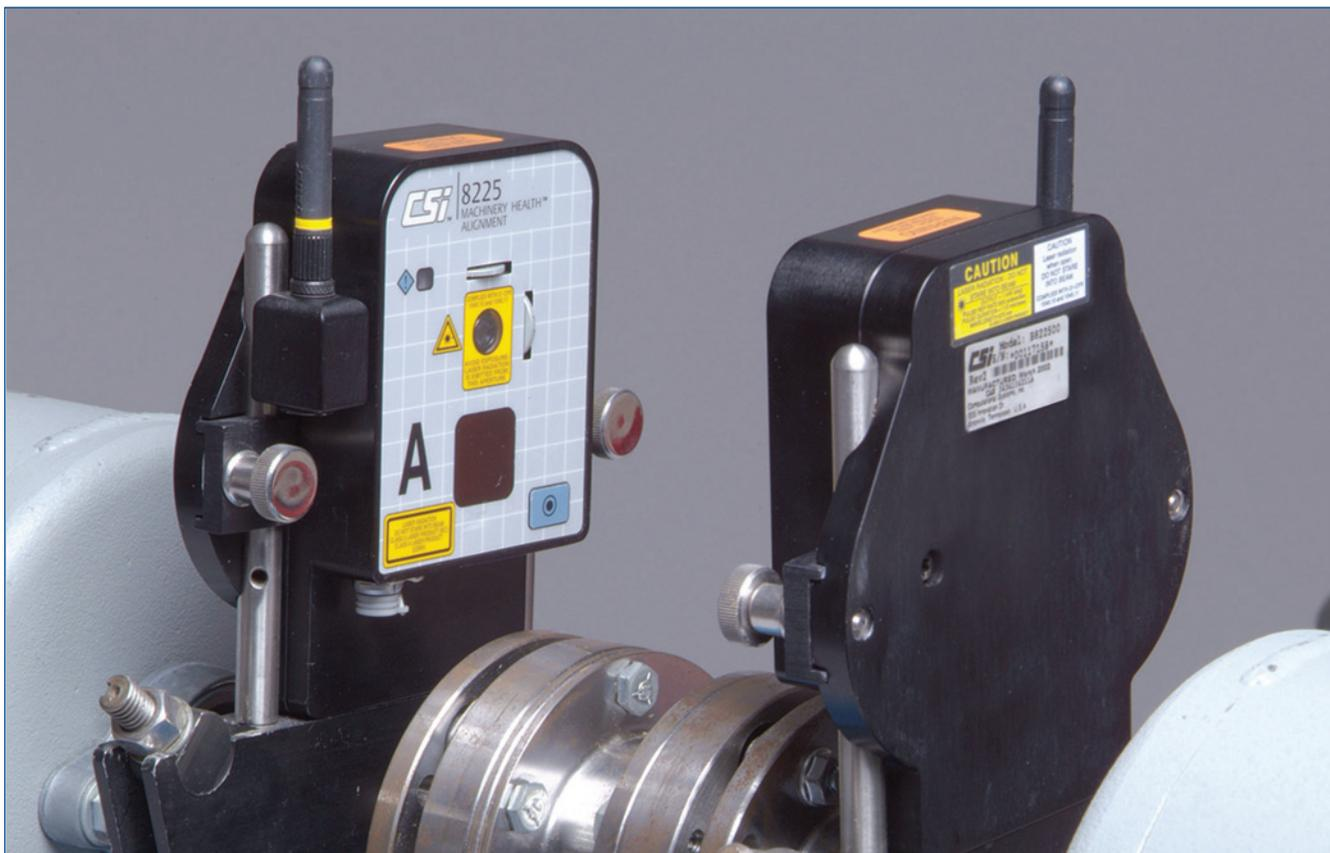
*Emerson's uniquely-designed laser heads and extensive accessory offerings create an alignment solution that is applicable to a wide variety of alignment jobs.*
