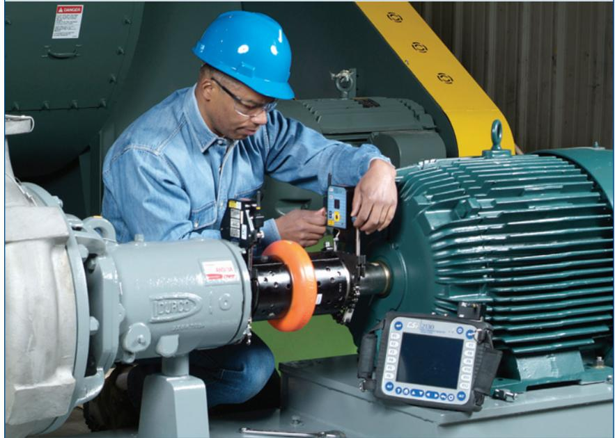
Adding laser alignment and dynamic balancing to your existing vibration analyzer creates a complete solution for your rotating machinery.
