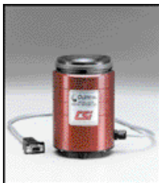
The 52DV digital viscometer uses a rotating ball to measure the viscosity of the oil sample.
