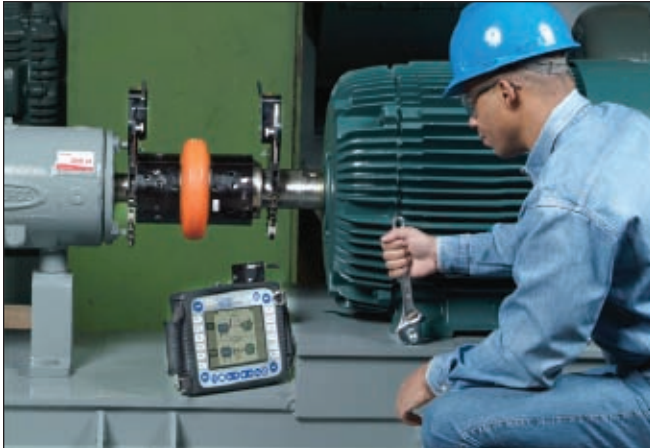
Laser alignment and precision balancing jobs can be stored and reported in AMS Machinery Manager.
